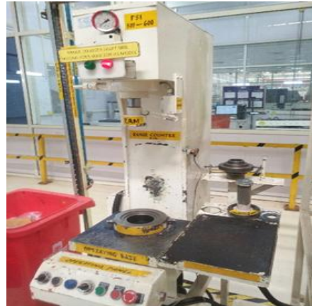
Fig .1 poka-yoke for needle roller bearing
